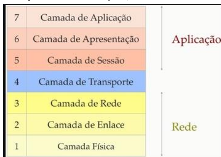
Figura 2 – Modelo OSI ( Open Systems Interconnection )
